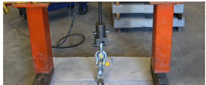
Figure 4: 1FA045 Foot Anchor tested in tension.
