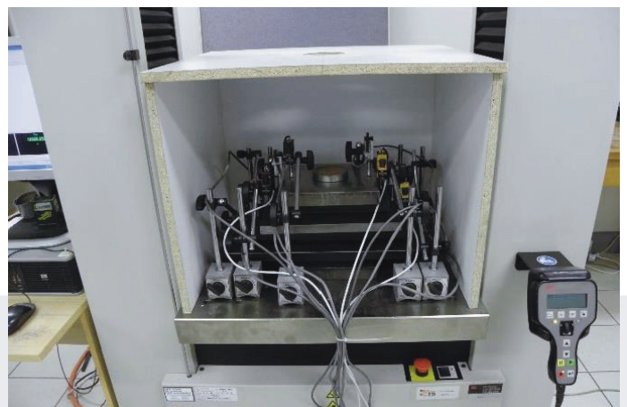
Figure 6: Test setup used for elevated temperature compression test
