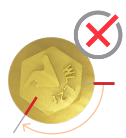
D - Greater than 90° Report to authority on site.
